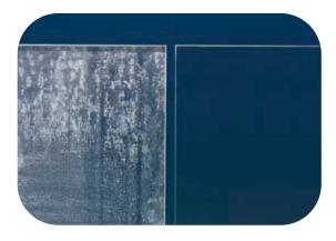
Aging tests at high temperatures and humidity demonstrate that Pilkington **OptiShower**<sup>™</sup> limits the corrosive process and limescale deposits compared to untreated glass.
